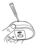
3. If necessary it is possible to further secure or tamperproof the alarm by using a No.2 or No.4 3/32 to 7/64 in (2 to 3 mm) diameter - not supplied self-tapping screw 1/4 to 5/16 in (6 to 8 mm) long to firmly lock the alarm and its mounting plate together.
