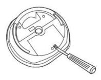
To remove the alarm once installed, it is now necessary to use a small screwdriver, to release the catch (push catch towards the ceiling) and then twist off the alarm.
