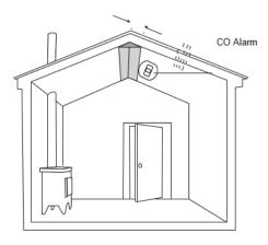
Note: The CO Alarm should be located at the high side of the room.
