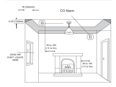
Figure 2: CO alarm in a room with sloped ceilings
