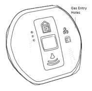
Within seconds, the red LED begins to flash (as per Table 2) confirming that the alarm has detected the CO.
